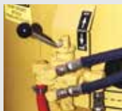
FWD/REV Hydraulic Agitation Valve
