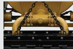
Dual Easy-Open Butterfly Sealer Discharge Valves
