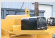
Anti-Splash Material Loading Hatch
