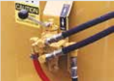
Forward / Reverse Full Sweep Agitation
