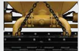
Dual Easy-Open Butterfly Sealer Discharge Valves
